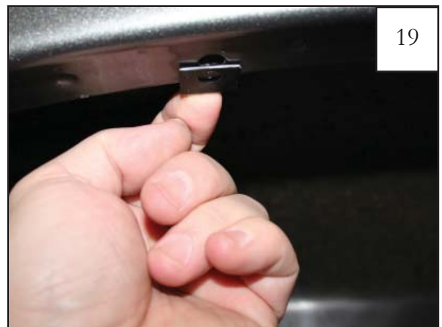
Install Clip (CL1-0022) over existing hole.
