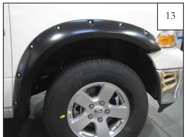
Completed front flare installation.
