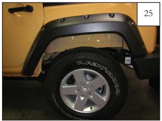
Ensure fit, and tighten all screws
