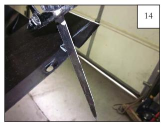
On rear end of splash sheild using a grease pencil, measure in from last hole 1-1/4" and make a line from the edge of shield to style line. Then create a line from the style line out to the end of the splash sheild as shown. Using sawsall to cut off section marked.
