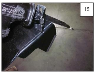
On front end of splash sheild using a grease pencil and mark in 1/2" from the radius of splash sheild and drawn a line till flush with outside edge of shield. Using a sawsall cut off section of splash sheild where indicated.
