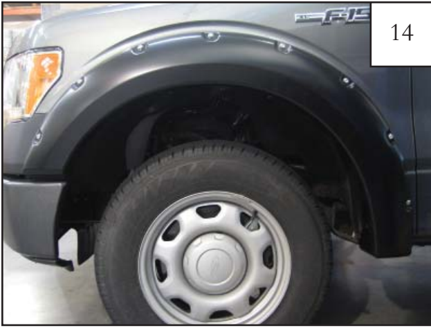
Completed front flare installation.
