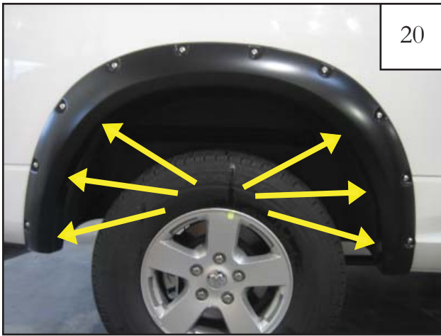
Hold flare in place while you start six factory screws using an 8 mm socket wrench. Do not tighten.
