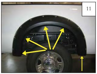
Ensuring proper flare placement, tighten all screws.
