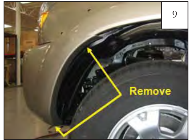
Remove two factory screws from front bumper fender extension. Save screws for reinstallation.
