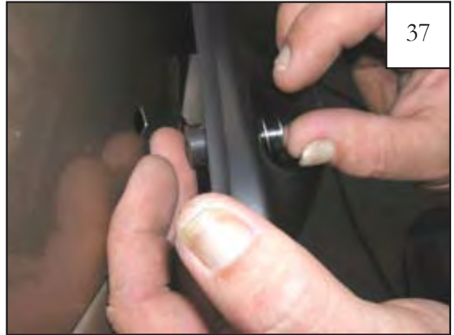
Install Screw/Washer assembly through foremost pocket hole in the Front Main Flare. Place a supplied Spacer (SP1-0011) on the back of the screw. Remaining pockets will use Screws (SW1-0032). Steps 2 - 3.
