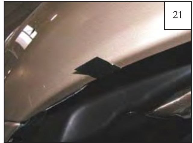
Removed flare from fender. Stick a supplied Tab (MT1-0002) over marks made in step 19. 4 places.
