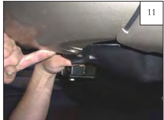
Pull down bumper cover and splash shield.
