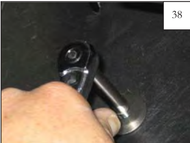
Pull back splash shield. Install a supplied Washer (WA1-0017) and a supplied 8 mm Serrated Flange Nut (NU1-0011) on back of screw. Tighten.
