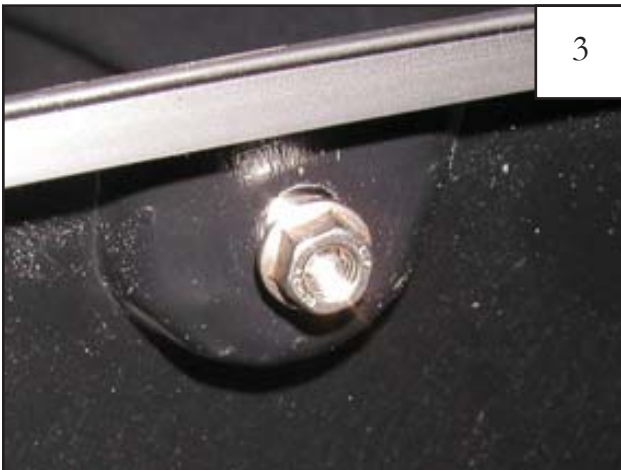
FRONT MAIN & REAR FLARE ONLY: Place a Nut (NU1-0019) over the end of each Bolt and tighten, using a 1/2" wrench for the Nut and the supplied Torx Bit (SW1-0052) for the Bolt. Repeat for remaining pockets.
