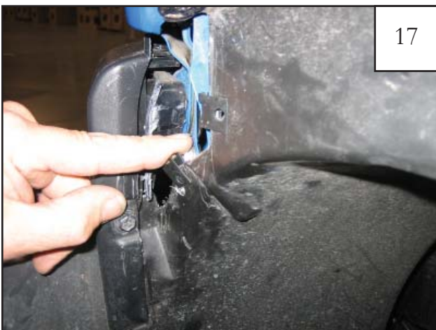
Slide supplied Clips (CL1-0022) over holes drilled in previous Step (2 places).
