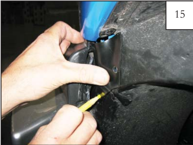
Holding Front Inner Piece on front of wheel well next to bumper, use a grease pencil to mark two clip locations.
