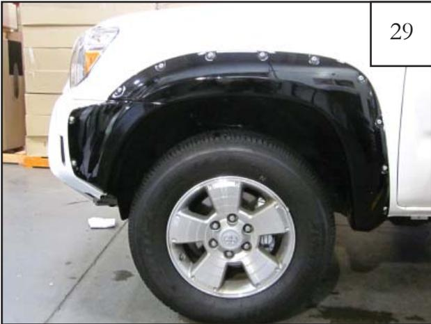
Tighten all screws. Completed Front Flare installation
