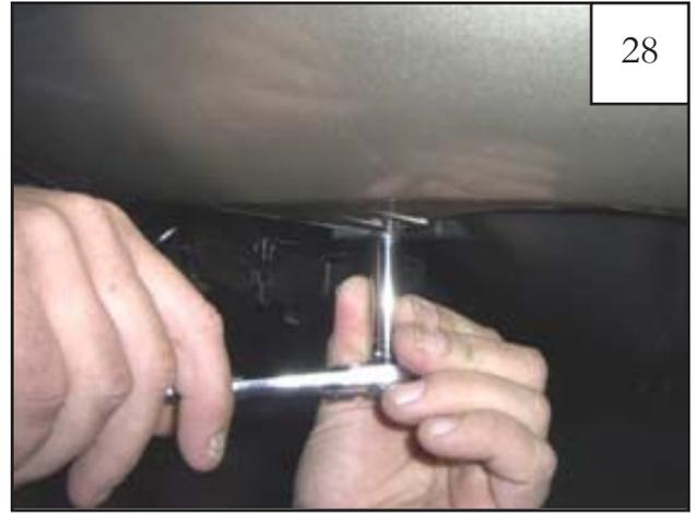
Pull down bumper cover and slide splash shield back in place. Install supplied hex screw (SW1-0036) in front of bumper cover to fasten splash shield to bumper
