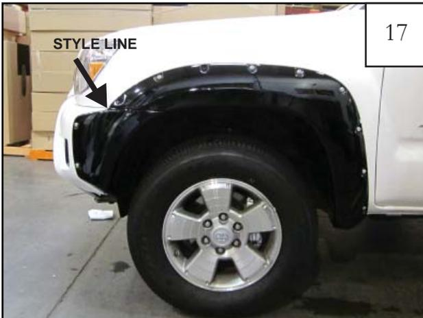
Hold the flare firmly on the fender. Make sure to line up the flare and bumper piece along the style line to ensure correct installation.
