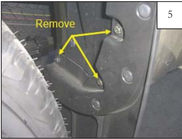
Remove three factory screws from mud flap. Discard mud flap.
