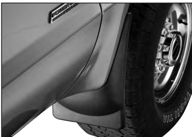
**10** Begin passenger side installation by parking the vehicle on a level surface with the wheels turned fully to the right. Repeat steps 3-9.
