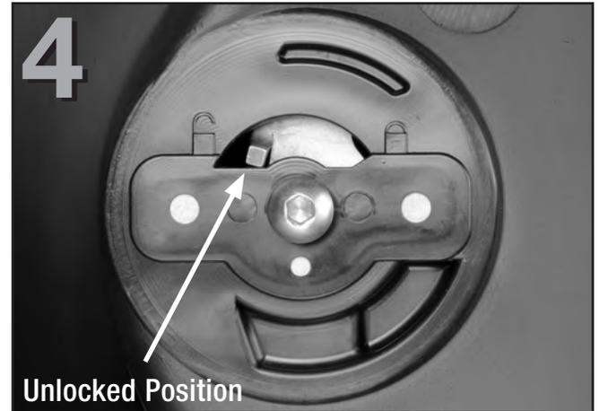
Identify the driver's side MudFlap by locating the "LH" mark located centrally in the recessed cavity on the tire side of the MudFlap. Ensure that the QuickTurn™ fastener is in the fully unlocked position using the Allen wrench provided.
